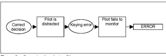
Figure 3 Example of an Action Slip
