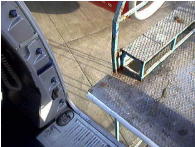
Large gap between aircraft and gantry caused by high winds buffeting the aircraft
