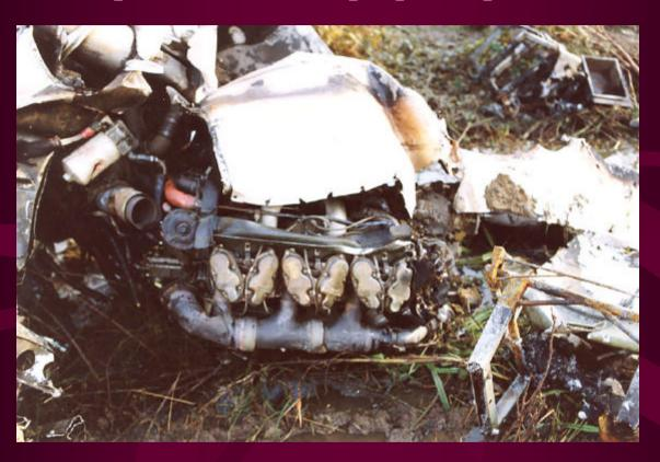
Severe ground fire precluded positive identification of left engine problem, but possible rough running due to problem with aneroid unit in fuel pump identified
